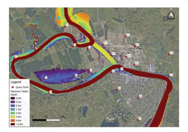
Option 1B is also a variation of Option 1 and involves a 1km floodway measuring 170m wide and 2m deep, with 1m high stopbanks on either side. This option would also provide effective flood mitigation to much of North Clyde as it would create a concentrated flow path for excess water flow.
