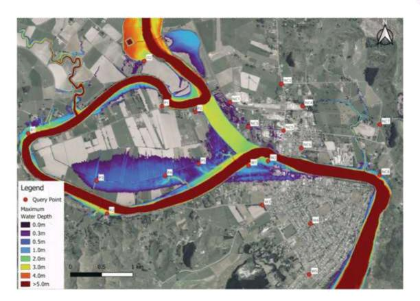
Option 1A is a variation of Option 1 and involves a 1km floodway measuring 250m wide and 2m deep, with no stopbanks. This option would provide effective flood mitigation to much of North Clyde as it would create a concentrated flow path for excess water flow.
