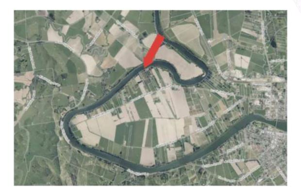
Option 7 involves constructing a new river channel or spillway to move flood waters away from the North Clyde area where the banks breached in Cyclone Gabrielle. With this option, significant flooding still remains in North Clyde.
