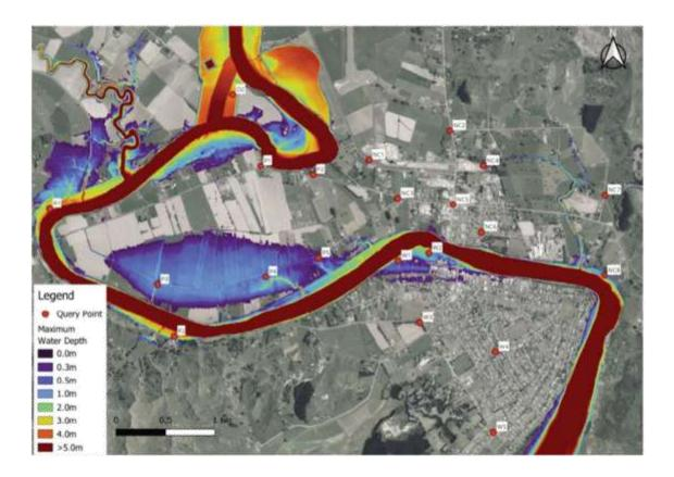
Option 17 was a combination of the stopbank of Option 5, with the addition of Option 7 which involves a 600m long and 2-3m deep floodway to reduce flood impact to Huramua. This combined option negates some of the negative effects of option 5 by providing marginal storage, however negative impacts for the Huramua side remain.
