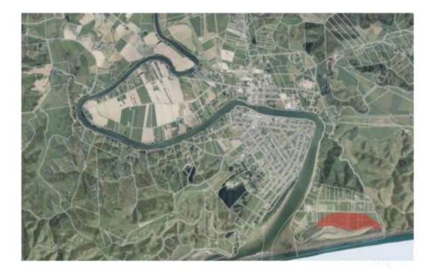
Option 13 involves extending Ngamotu Lagoon near the river mouth to provide additional flood storage detention. This option provides no notable flood reduction for North Clyde.
