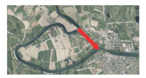
Option 1 is a flood spillway, which would only be used when river levels are high enough. This option may need stopbanks along each side to prevent overtopping and drains for stormwater run-off when not in use. This option would provide effective flood mitigation to much of North Clyde as it would create a concentrated flow path for excess water flow.
