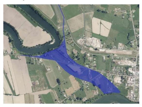
**Option 1C is one of the two most technically viable flood mitigation options which require further consideration.** This option provides effective mitigation for much of North Clyde as it creates a concentrated flow path for excess water flow. This option also performs better than Option 1D as it protects more area and has very few negative flood impacts.
