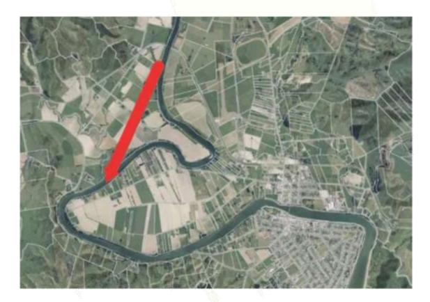
Similar to Option 7, Option 8 involves constructing a new river channel or spillway to move flood waters away from the North Clyde area where the banks breached in Cyclone Gabrielle. With this option, significant flooding still remains in North Clyde.
