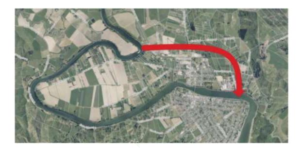
Option 4 involves constructing a new spillway to redirect flood waters around the township of Wairoa and toward the Awatere Stream. This option would provide some reduction of flood depths within some areas of North Clyde, but is a less hydrologically efficient floodway than Option 1.
