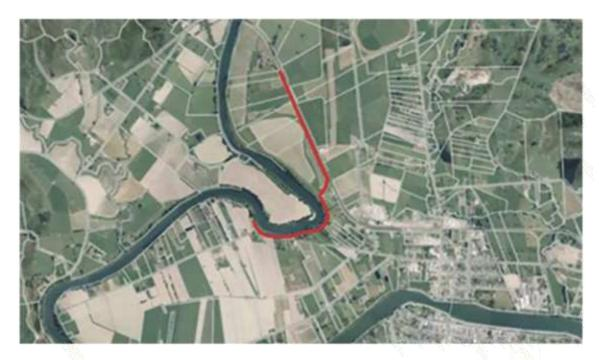
Option 5 aims to keep flood waters within the channel and involves the construction of continuous stopbanks along the Wairoa River. This option would provide effective mitigation for much of North Clyde, however additional flooding occurs on the Huramua side of the bank, State Highway 2 (SH2) and along Ruataniwha Road. This option also creates water level increases within the main river channel back to Frasertown.
