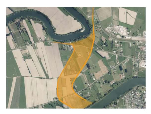
Like Option 1C, Option 1D is the second of the two most technically viable flood mitigation options which require further consideration. This option also provides effective mitigation for much of North Clyde as it creates a concentrated flow path for excess water flow, however it doesn't protect as much land as Option 1C.
