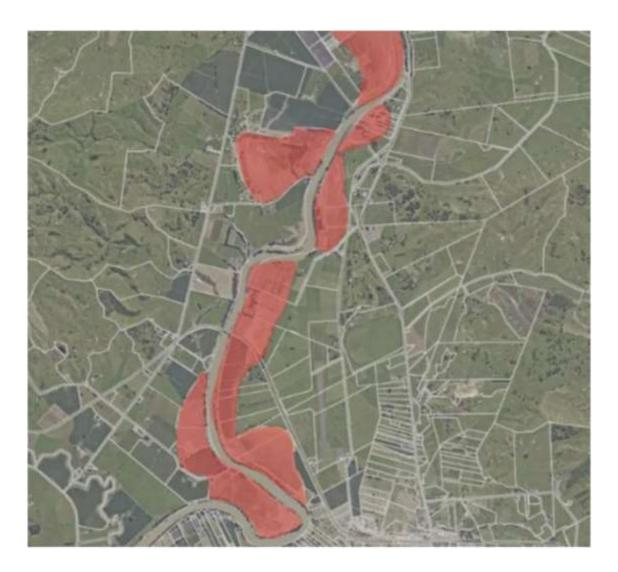
Option 3 involves using old flood plains and historic river oxbow lakes as flood storage detention. This option would provide no notable flood reduction for North Clyde.
