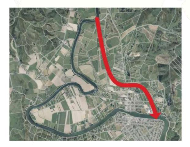
Similar to Option 4, Option 6 involves the construction of a spillway to redirect flood waters around the airport and North Clyde area, via existing drains and the Awatere Stream. This option does not mitigate enough flooding and is a less hydrologically efficient floodway than Option 1.
