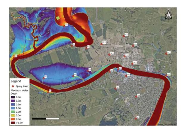
Option 5C is a variation of Option 5 and involves 5.3km of stopbank around 2m in height but up to 4m in height in some places, aligned to existing road corridors where possible. This option would provide effective mitigation for much of North Clyde, however additional flooding occurs on the Huramua side of the bank, State Highway 2 (SH2) and along Ruataniwha Road. This option also creates water level increases within the main river channel back to Frasertown.
