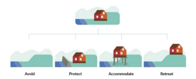
Option 16 involves raising the finished floor level of houses to prevent damage during flooding. In some instances, armouring of the foundations may be required.
