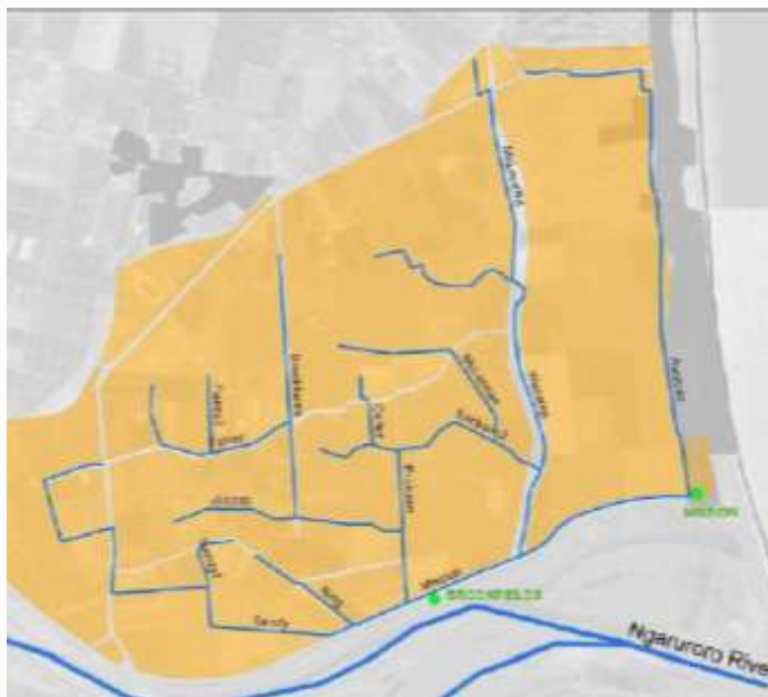
Figure 1b: Brookfields/Awatoto Scheme showing Napier Urban stormwater drainage area with open waterway and pump station locations and names
