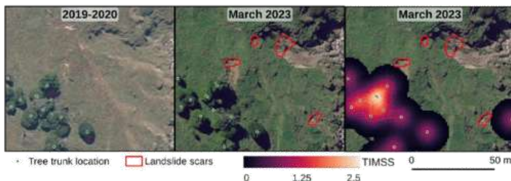
Figure 2. Illustration of spatial application of the TIMSS . Multiple landslides occurred during the Cyclone Gabrielle, which can be seen on March 2023 imagery, compared to previous one. Although trees contribute to slope stability, they do not always prevent landslide erosion – a reflection of a multivariate problem. Note that the influence of more than one tree at a given location is assumed to be additive, which is why values exceed 1.
