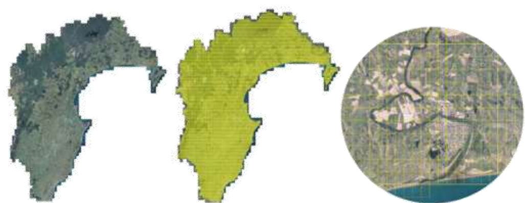
Figure 2. Aerial LiDAR data in Hawke’s Bay. (Left) Full coverage; (Middle) Individual LiDAR tiles shown in yellow; (Right) Zoomed-in view as example over Wairoa.
