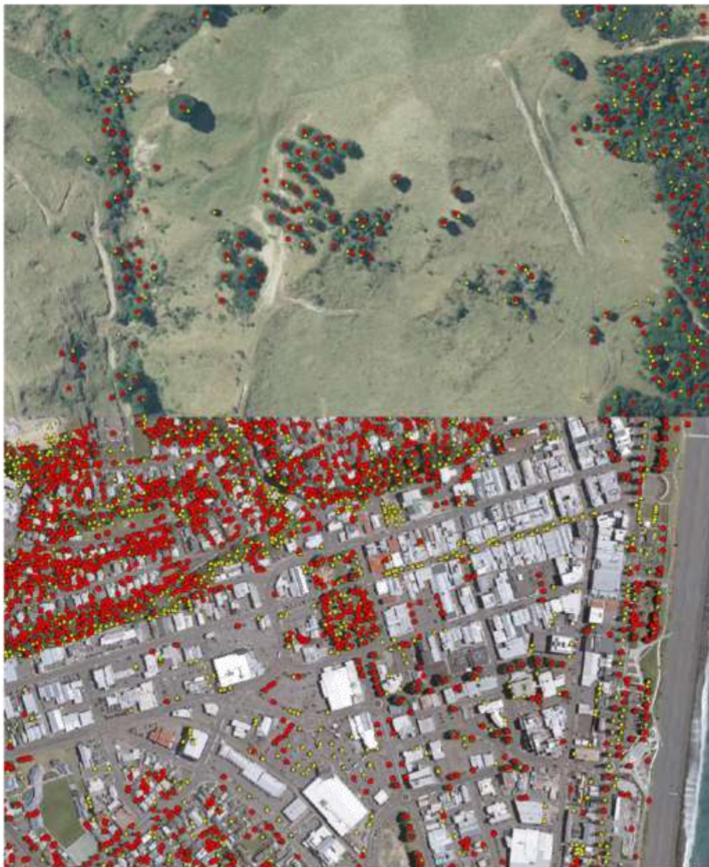
Figure 29. PyCrown LiDAR-derived tree locations (red dots) vs YOLO deep learning estimates (yellow triangles). (Top) Rural scene; (Bottom) Urban scene in Napier. The red PyCrown predictions are on top of the green YOLO predictions leading to some of the latter not being visible. PyCrown used a 3 m tree height threshold, whereas no height threshold was used in the image-based approach.
