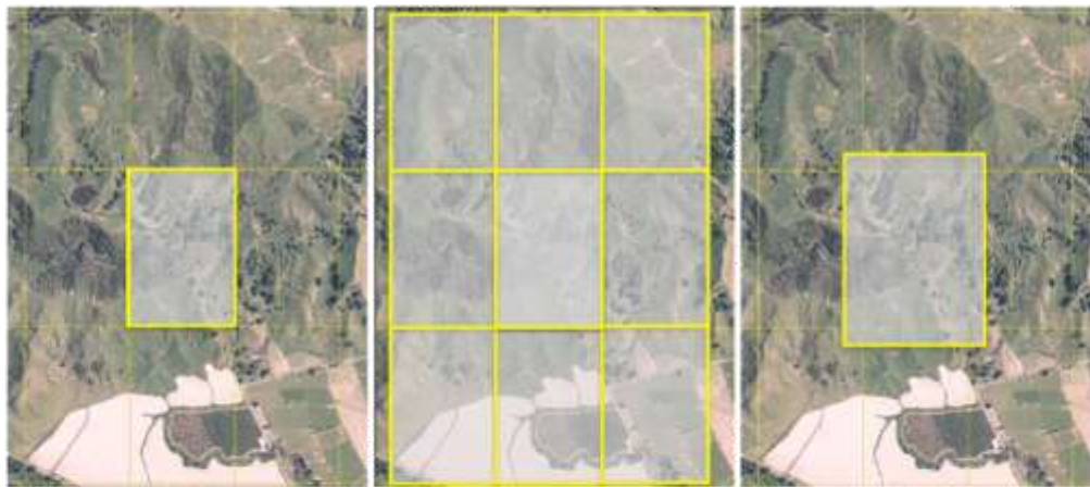
Figure 3. Creation of buffered LiDAR tile data. (Left) Original. (Middle) For each LiDAR tile, the eight neighbouring tiles are merged; (Right) The merged tiles are then clipped to the central tile extent with a 60 metre buffer area.
