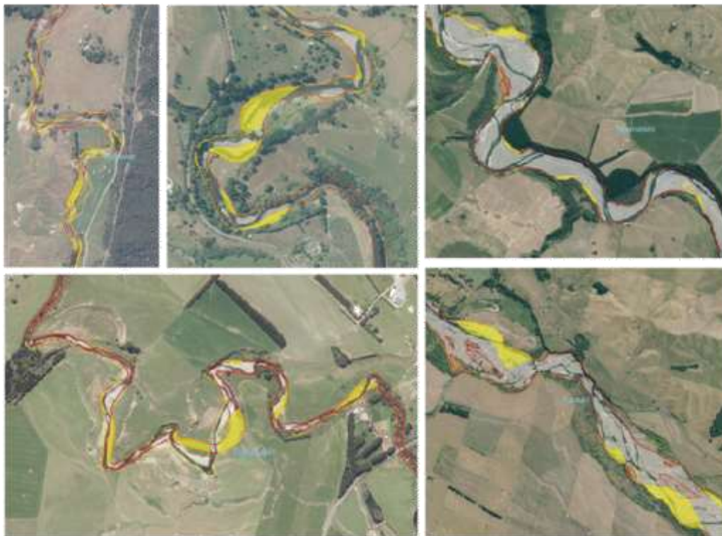
Figure 7. Examples of channel planform mapping showing areas of erosion (yellow shading) with mapped channel banks from 2010–11 (yellow line) and 2019–20 (red line) aerial imagery.
