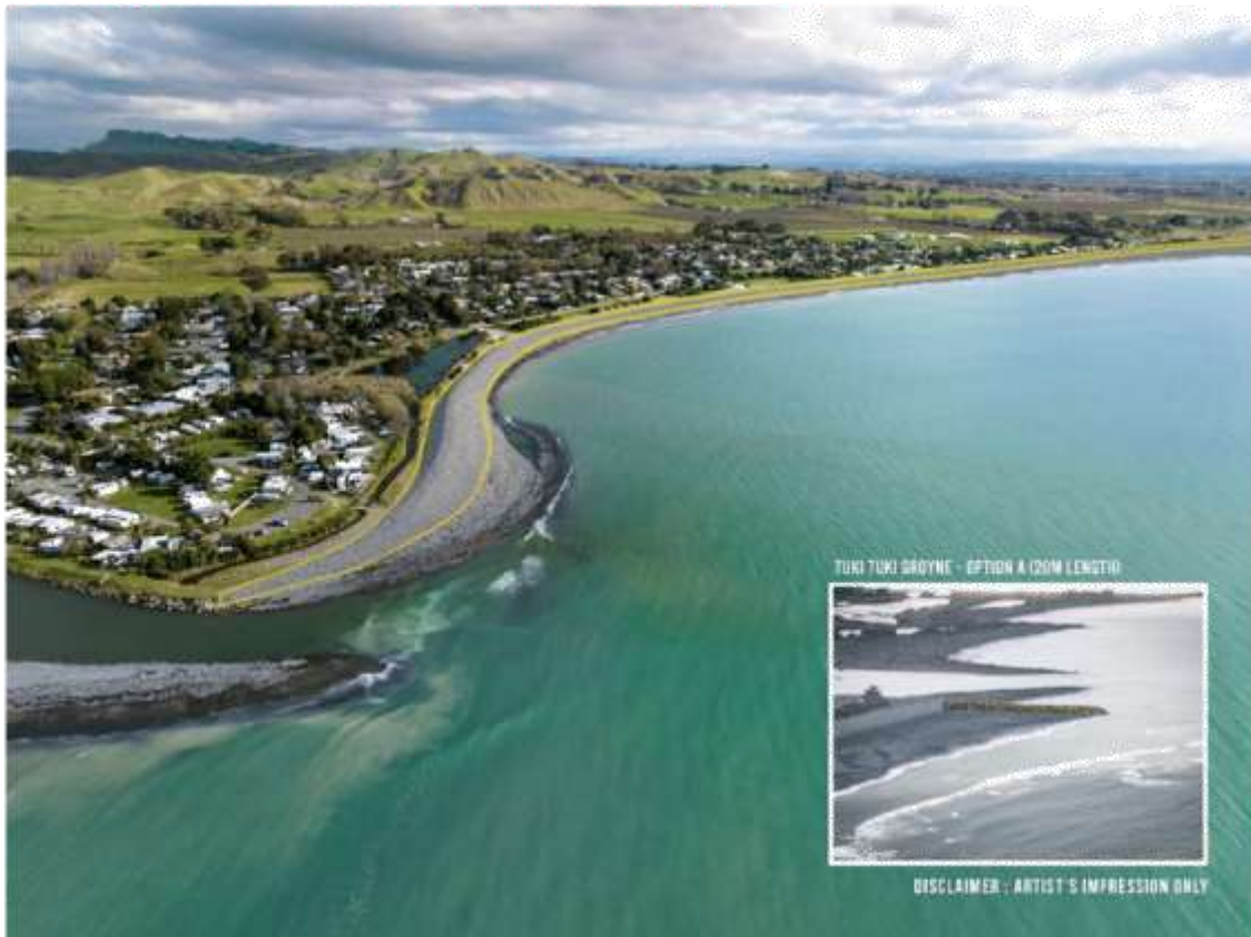
Figure 18: Te Awanga Pathway Action (Option A) indicative location of proposed on-shore gravel nourishment with single groyne further north at Tukituki River mouth
