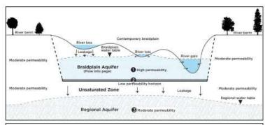
Hydraulically connected (recharge lateral)
