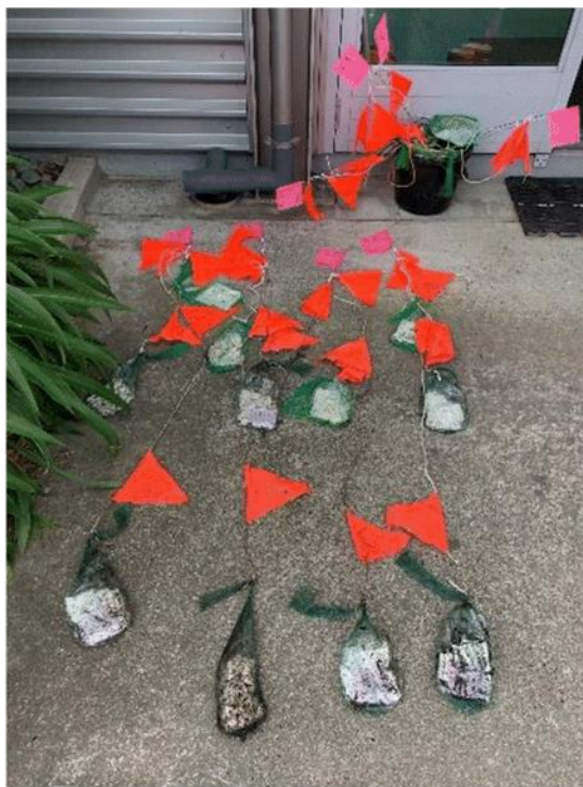
Figure 3. Vacuum-sealed bags inside netlon mesh bags after they have been buried in compost for 1 week.
