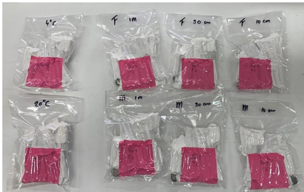
Figure 1. Vacuum-sealed bags containing 16 vials with pathogens and a temperature logger.
