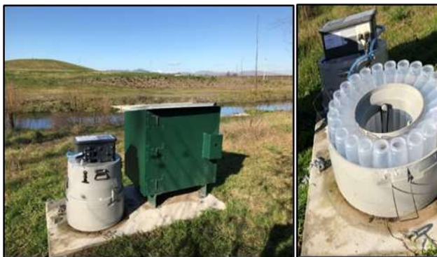
Figure 3: Automated sediment sampler (ISCO)
