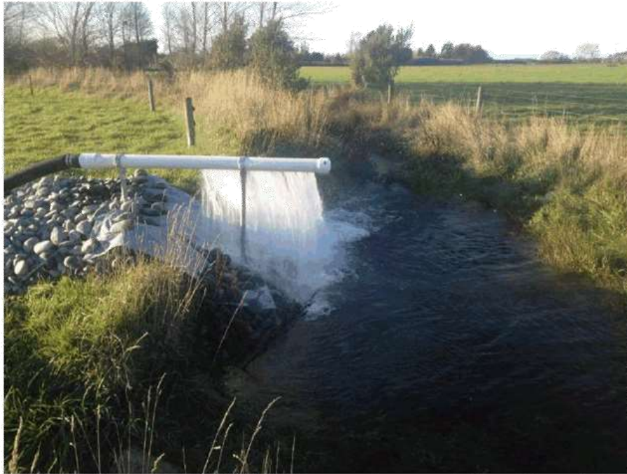
Figure 9; Discharge point of targeted stream augmentation trial in Boggy Creek, Canterbury. Water is supplied through multiple holes in the PVC pie and discharged on to cobbles to increase the dissolved oxygen content.
