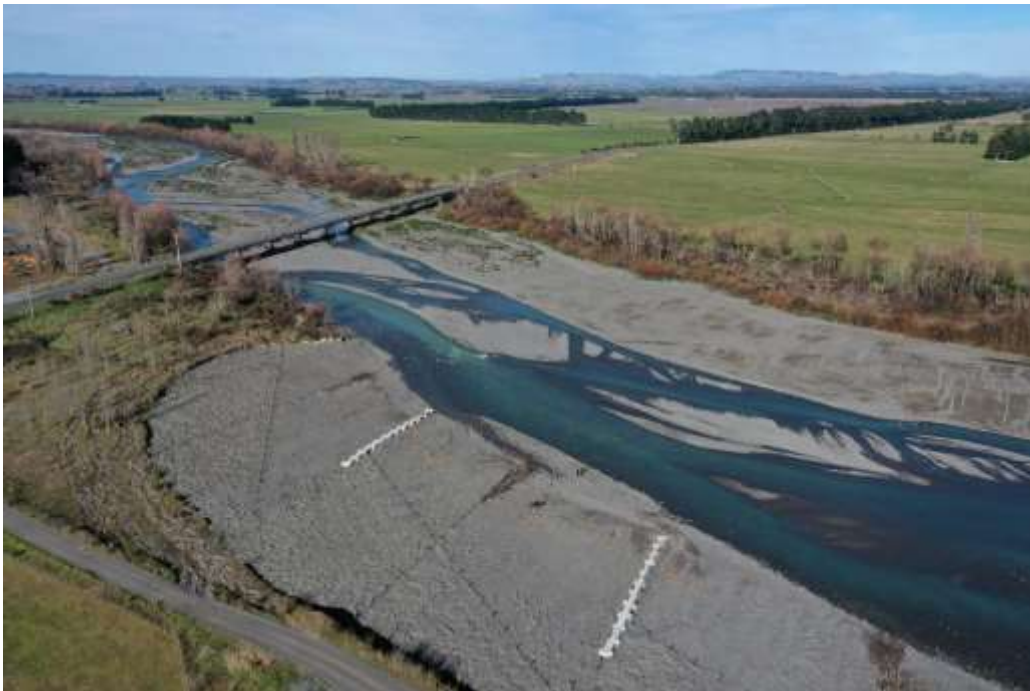
Photo 1 – Akmon and rope and rail features on the true left bank of the Waipawa River
