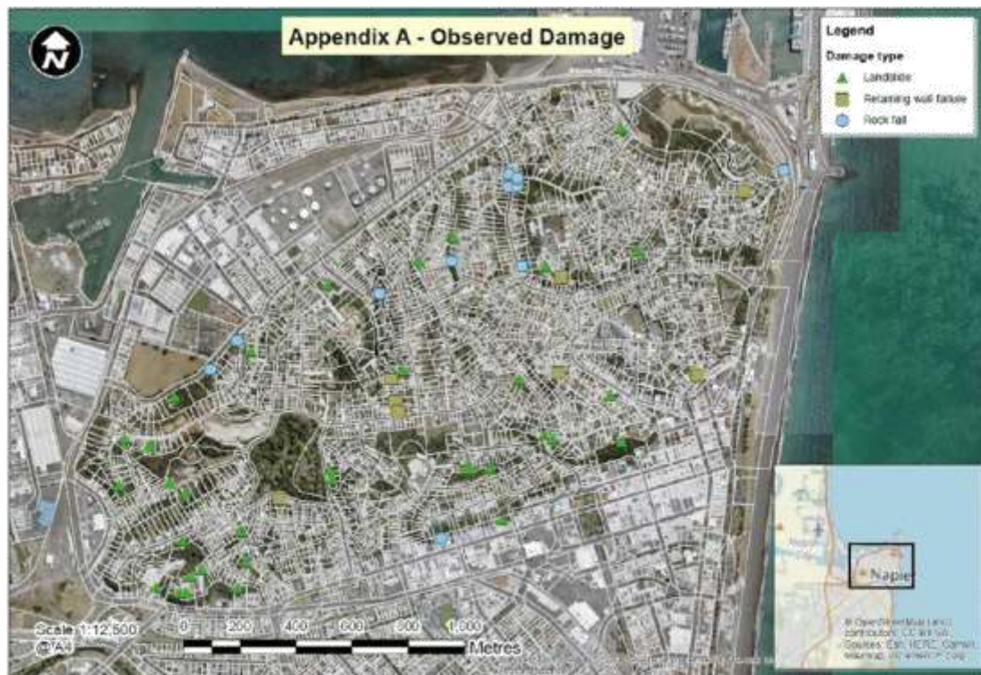
Figure 80: Observed damage on the Napier Hill, taken from WSP Engineering Reconnaissance Report, 12th November 2020
