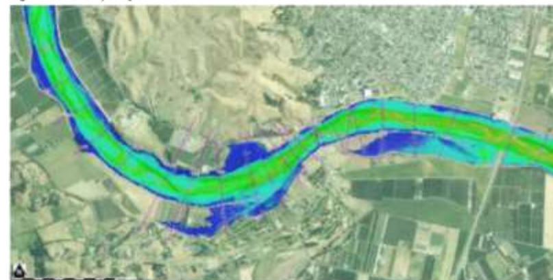
Figure 20: Example of a Flood model scenario on the Tūtaekurī River at Taradale
