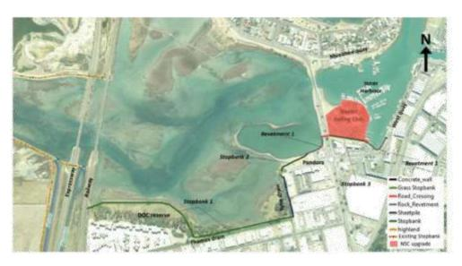
Figure 10: Layout design for the proposed flood defences in the Pandora Priority Unit (Beya and Asmat, 2020).
