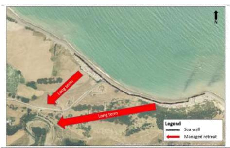
A 480m long reventment was recently repaired and constructed as part immediate steps to address coastal erosion in this area. To complete the short-term pathway, a further 630m is required to be constructed either side of the existing structure (Figure 22).
