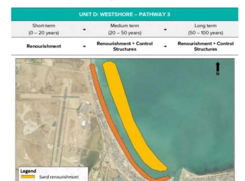
Further modelling and engineering concept design for this priority unit has identified that in the short-term, renourishment is likely to comprise of a combination of both sand and gravel renourishment as well was the extension of the existing gravel barrier at Westshore (Beya and Asmat, 2019).
