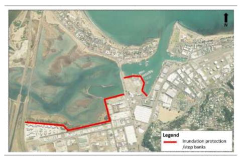
Further modelling and engineering concept design for this priority unit has identified that in the short-term, a range of inundation protection measures will be required reflective of the broad ranging environmental settings along the proposed feature. This includes stopbanks, revetments and sheet pile walls. The composition of the inundation protection features is shown in **Figure 10**.
