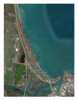
Figure 7: Approximate areas of the Westshore priority unit were an extension to the existing gravel barriers is required (Beya and Asmat, 2019).
