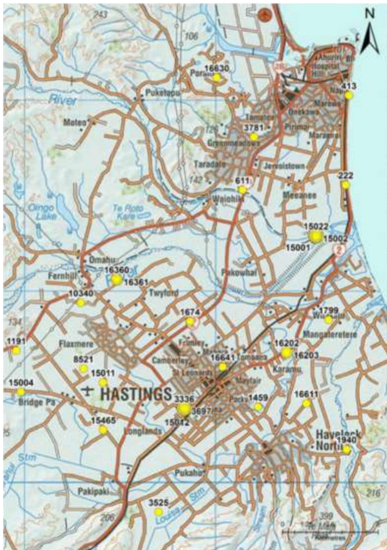
Figure 3-3: Heretaunga Plains bores used for monitoring groundwater quality. Bore numbers are shown next to yellow circles that show the location.
