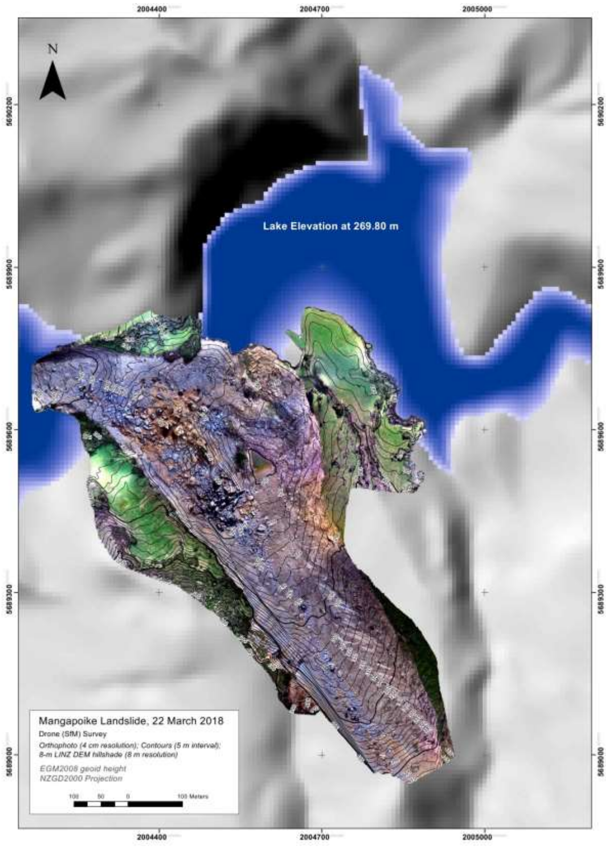
Figure 4: Aerial photograph of the landslide dam on 22 March 2018
